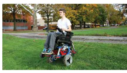
Six independent, height-adjustable wheels allow MEBot to adjust to different terrains.
